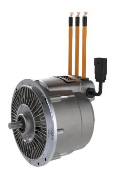
integrated with Omni planetary or parallel shaft gearboxes to sustain continuous torque ratings to 7000 Nm. These motors are suitable for a range of voltages from 24V-96V, feature an IP67 rating, and can be supplied with a range of brake and encoder options.
