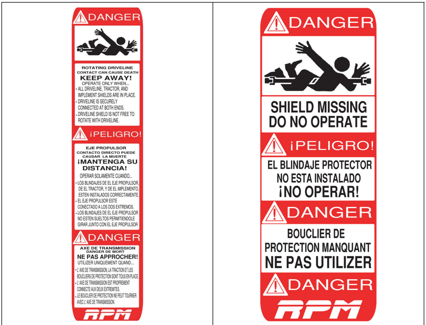
Figure 1. Driveline Shield Warning Label
