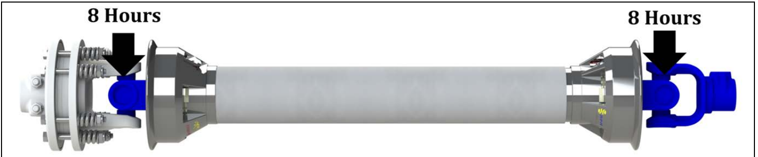
Figure 7. Universal Joint Lubrication Intervals
