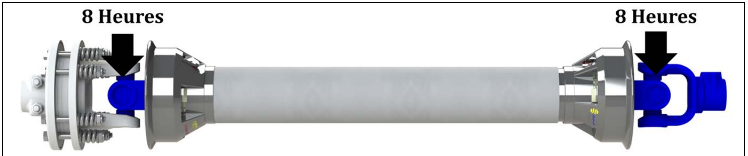
Figure 7. Intervalles de Lubrification des Joints de Transmission
